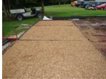
2. To measure decay rates a string was placed over the surface in three areas of the beds and a measurement was taken between the string and the top of the surface on the first day of installation in July of 2009. The beds were left to weather until April of 2011.
