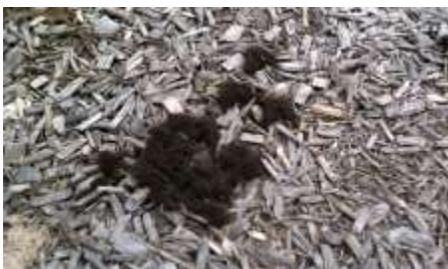
This is not to say that drainage will totally prevent mold and fungus from forming on the surface of EWF. Climate conditions, lack of sunshine and use will also effect the growth of molds on the surface of EWF but it was apparent that lack of drainage may have had something to do with the appearance of mold in just this one bed and not the other two.
