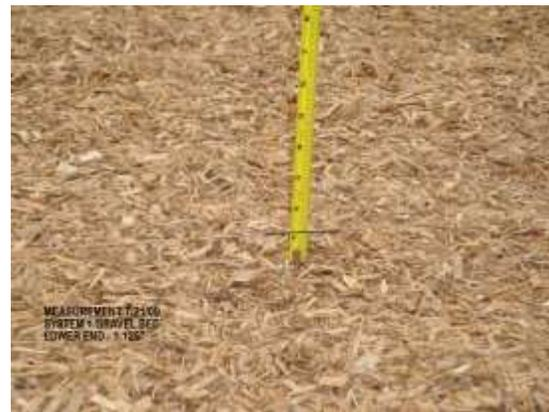
3. In April of 2011, the surface was compacted by using a hand tamper and dropping it approximately 24” from the surface.
